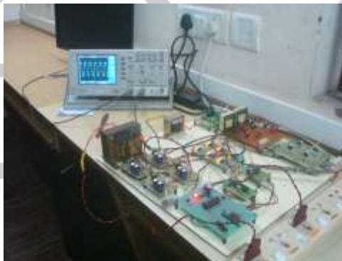
Fig 5.7 Hardware result of the high speed step up converter in DC-AC converter
