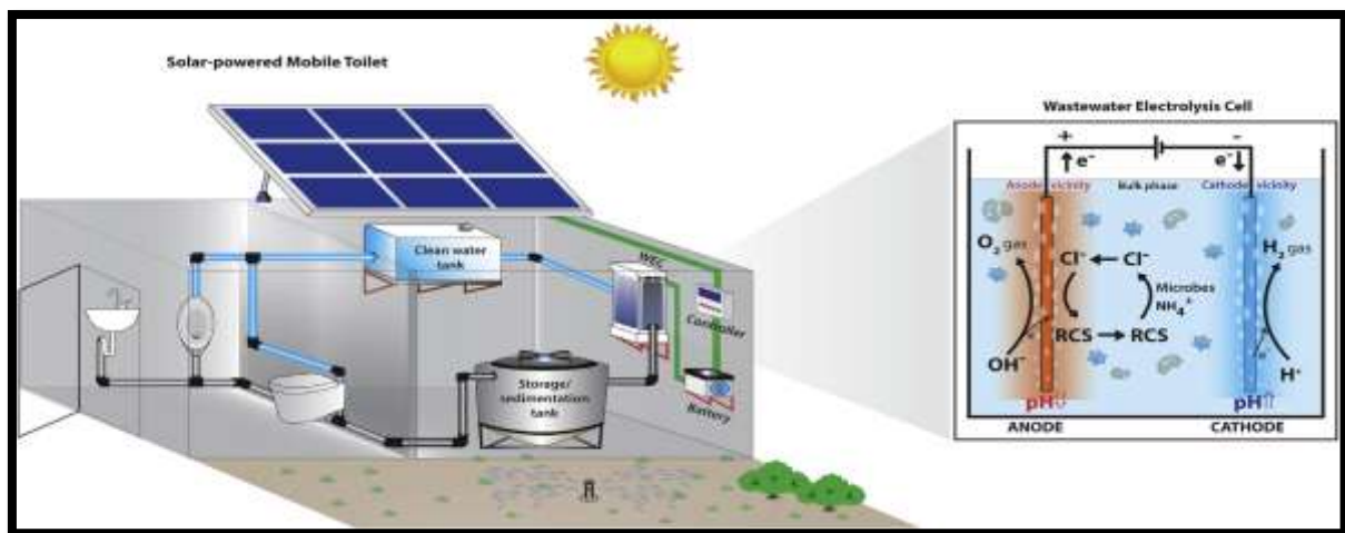
Fig.2. Schematic diagram of a solar-powered electrolysis cells for toilet wastewater treatment.
