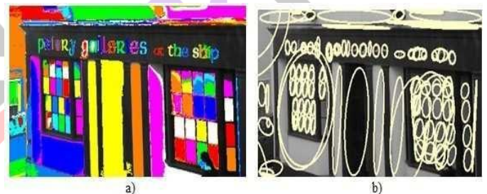
Figure 4. a) Output of detected regions as MSERs; b) Applying ellipses on detected region
