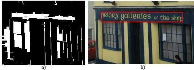
Figure 5. a) Output of morphology b) Output after the non-text elimination and text construction with rectangle.
