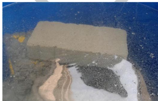
Fig. 10 Water Absorption Test
