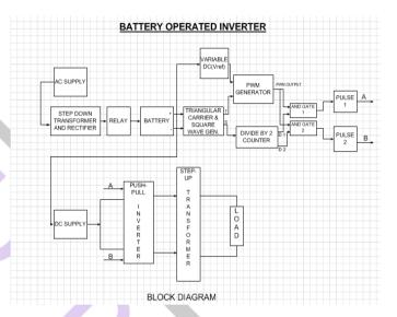
The ac supply is given to a step down transformer followed by a rectifier unit. The dc, so obtained is given to the relay COIL .The relay has 2 CO contacts. As per the relay operation, when ac supply is ON the battery is charged and supply is given to load. When the ac supply is OFF the battery gives supply to the inverter circuit and the output of it is given to the step up transformer and then fed to load.
