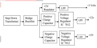
Rectifier units are usually capacitors acting as a surge arrester. This capacitor is also called as a decoupling capacitor or a bypassing capacitor.Regulator is connected to the DC output to maintain the voltage within a close tolerant region of the desired output. IC7812 and 7912 is used for providing +12v and -12v DC supply.
