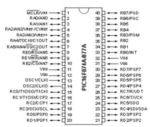
The microcontroller used here is PIC16F877A. The microcontroller has three 8-bit ports, one 6-bit port and one 3-bit port. It also consists of an 8-channel 10-bit ADC. The microcontroller is programmed such that the intensity is sunlight is measured at one
