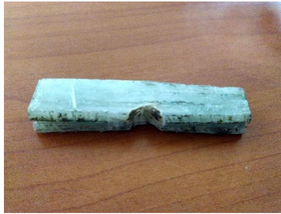
Figure 5 Fabricated Impact Test Specimen
