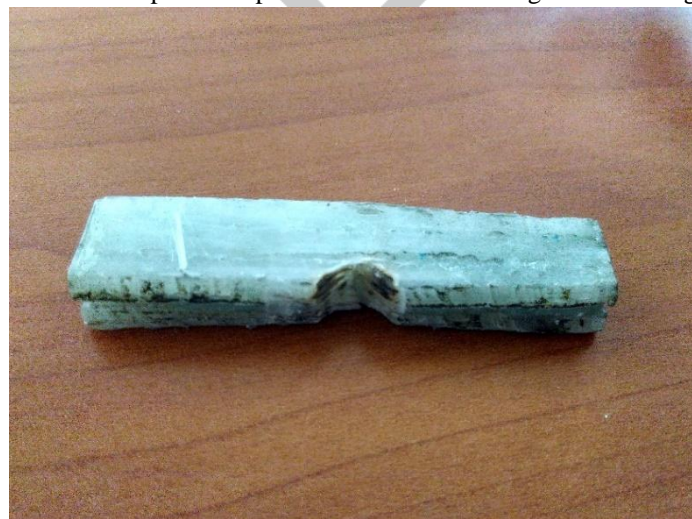
Figure 11 Specimen Before Impact Test
