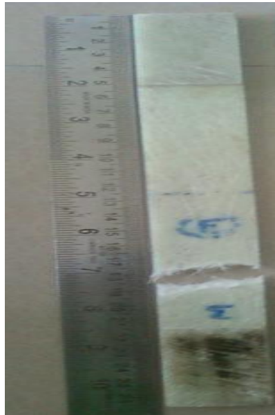
Figure 9 Specimen After the Tensile test
