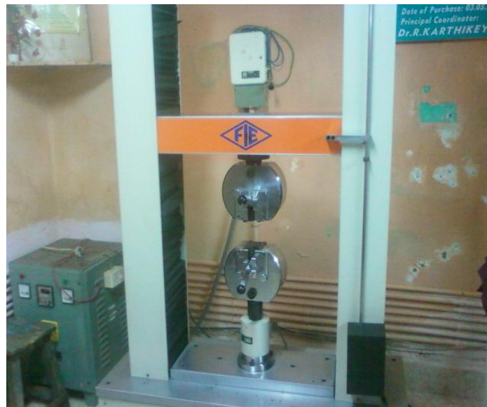
Figure 7 Tensile Testing Machine used for testing
