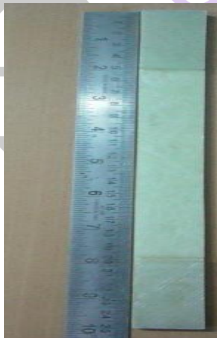
Figure 4 Fabricated Tensile Test Specimen
