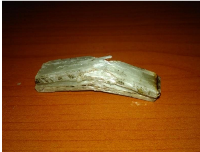
Figure 12 Specimen After Impact Test
