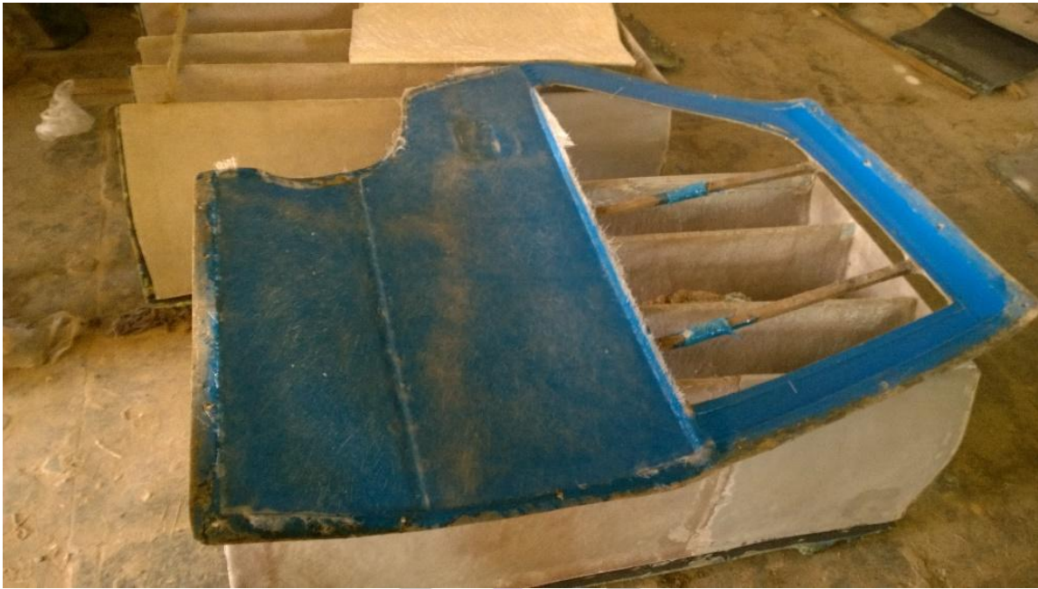
Figure 13 Mould for car door
