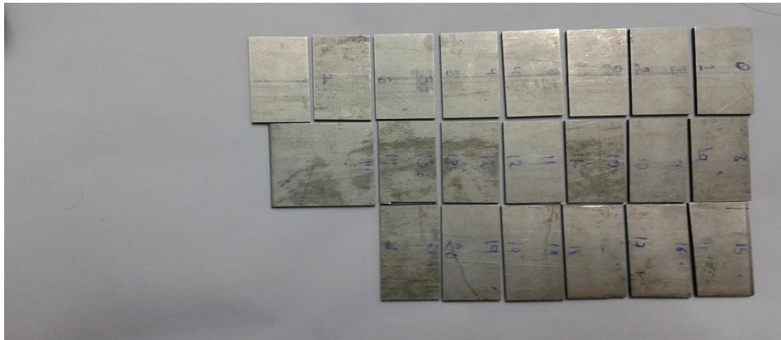
[Fig.4 cut out pieces by wire EDM]
