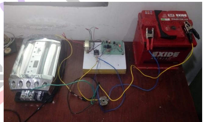
Fig.9. Charging of HUC using PWM technique
