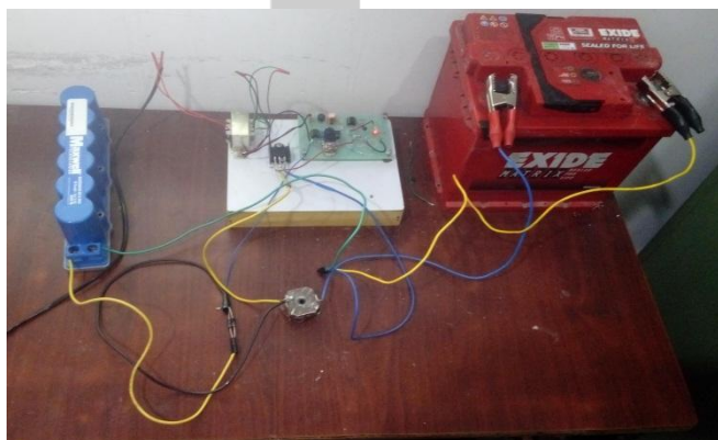
Fig.7. Charging of UC using PWM technique
