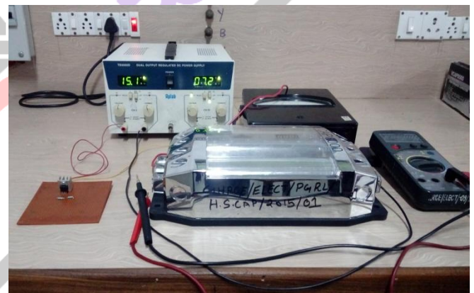
Fig.5. Charging of HUC using constant current method
