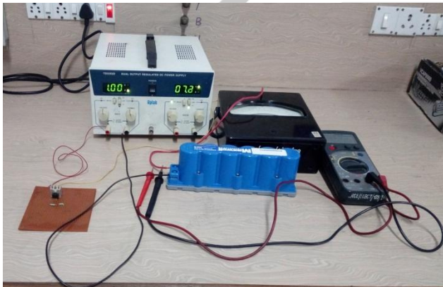
Fig.3. Charging of UC using constant current method
