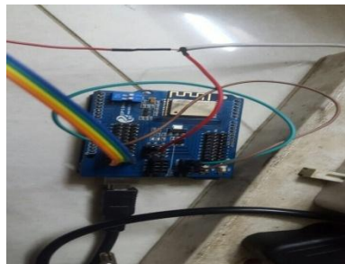
Fig 5.b: Assembly of Wi-Fi Module with Arduino UNO Board
