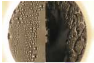
Fig 1.1 Filmwise & Dropwise Condensation
