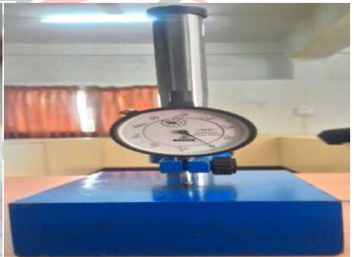
Figure 4 Dial Gauge Indicator
