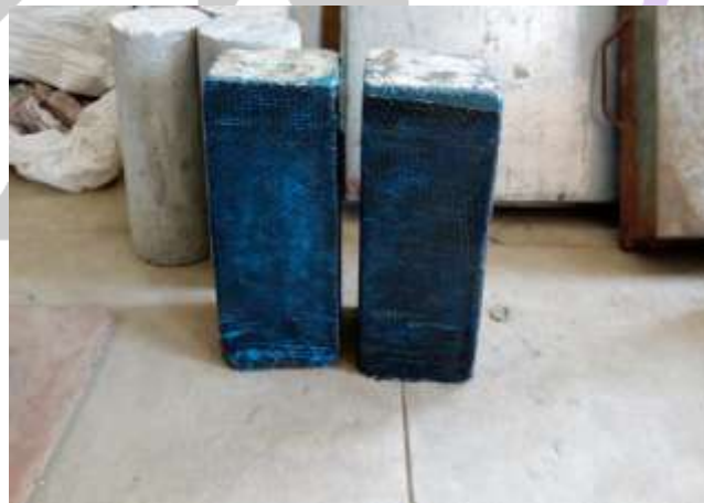
FIG 1: columns wrapped with CFRP sheet
