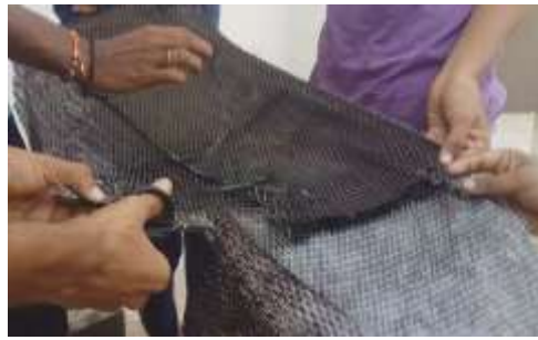
Carbon fiber cut with required size
