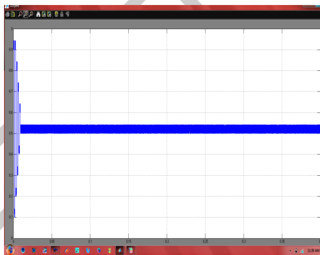
Fig.8 Waveform of the SB current during charging
