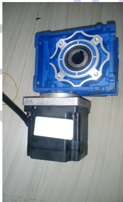
Fig. 4. Brushless DC Motor with Gear Box
