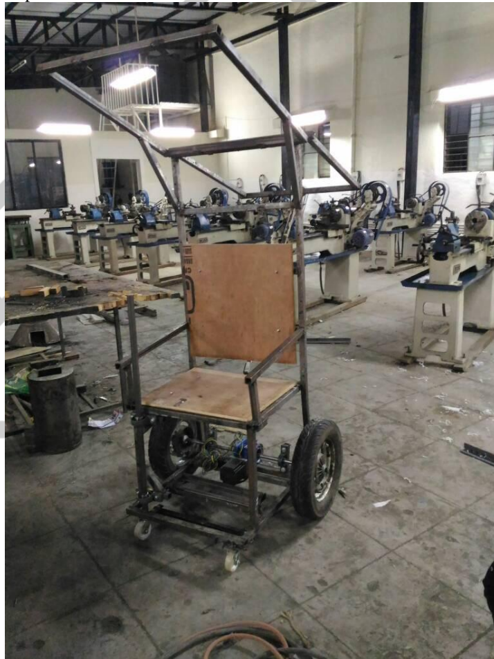
Fig.6. Designed Solar powered wheelchair
