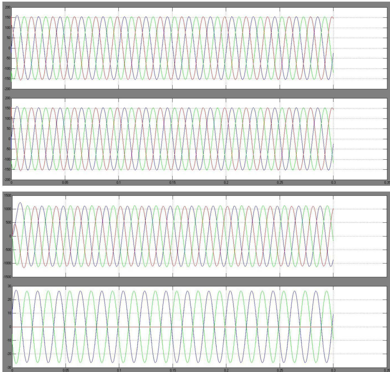
IUPQC transitory response during the connection of a two- phase diode rectifier: (a) load currents, (b) source currents, (c) load voltages, and (c) source voltages
