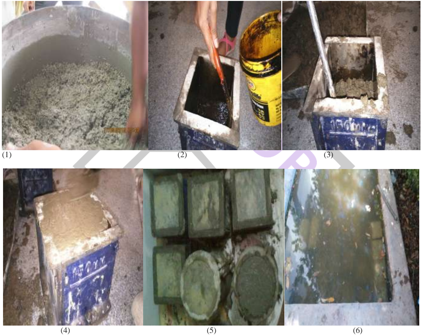
Fig. 1.2 shows the preparation of coconut shell concrete
