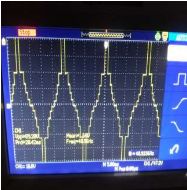
Fig 9.2 thirteen level inverter output
