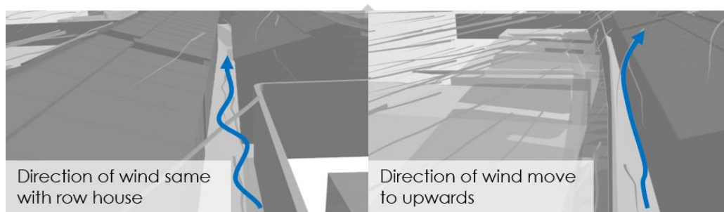
Figure 5. Airflow pattern in around building
