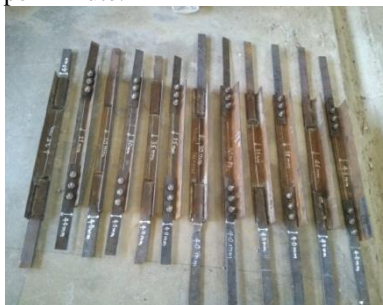
Fig 4 ISA Specimens with varying eccentricity
