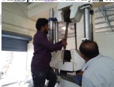
Fig 5 Specimen Clamped in UTM
