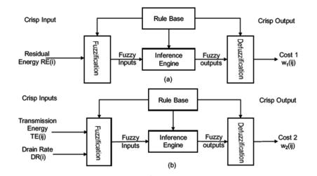
(a) Fuzzy System 1 (FS1) deals with the energy level related input. It takes the normalized residual energy or RE(i) of node i. It produces output variable RP1(ij), such that w1(ij) = 1/RP1(ij).
