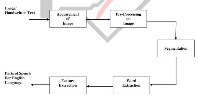
Fig: System Architecture of Real-Time Character Recognizer
