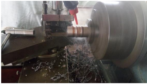
Fig 4. Turning process for 1.5mm depth of cut
