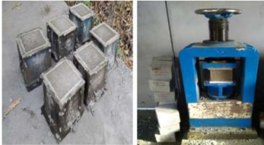
Compressive test of cubes
