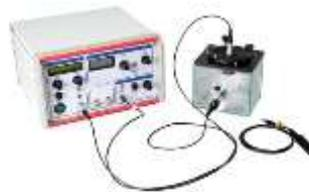
**Fig 1** – Ultrasonic continuous wave generator
