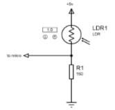
Figure 2: Light Dependent resistor
