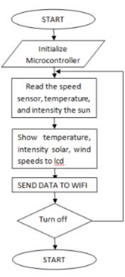
Figure 3: The Flow chart for the wireless based weather monitoring system
