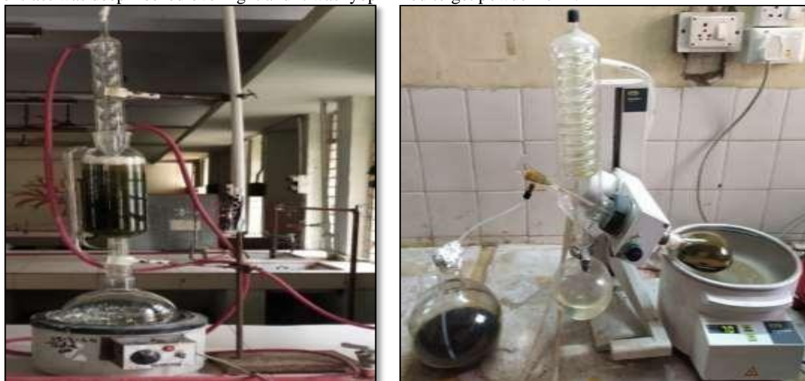
Fig.6.1. a) Soxhlet assembly during drug extraction b) Organic solvent evaporated using rotavapour.
