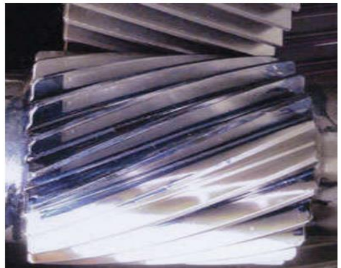
Figure 4 30% impressions formed on the adjacent gears
