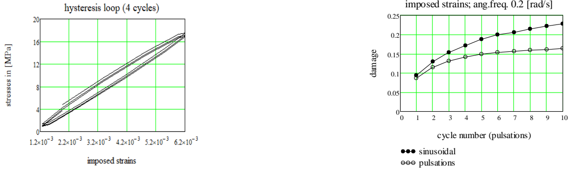
Fig.9 Hysteresis loops for 4 cycles – imposed pulsations Fig.10 Damage evolution in the case of two regimes
