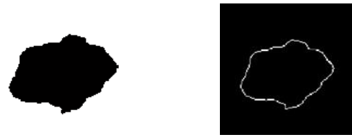
a) Area Open Image b) Boundary Image Fig 7. Edge Based Boundary Detection
