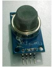
0.3 V; for higher concentrations, the voltage output reaches 4 V. The sensor board measures  $32 \times 20 \times 22$  mm and features 4 pins with 0.1 mm spacing **MQ7 Carbon monoxide sensor**
