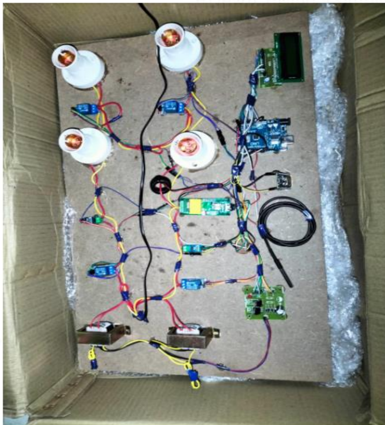
Figure 2: Hardware Kit of Load Balancing Using Load Sharing Technique In Distribution System
