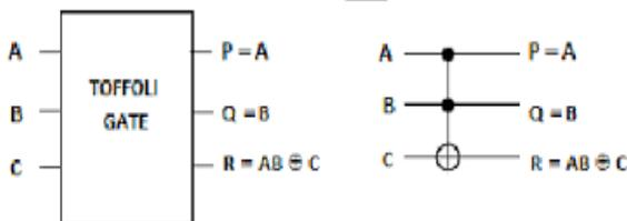
Fig 4 Operation and Quantum circuit of Toffoli gate
