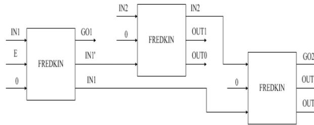
Fig 5(a). 2x4 Decoder using 3 FDK gates
