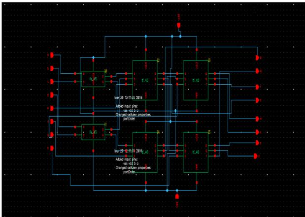
Fig 8. 2x4 Decoder using 2FEYNMAN & 4 TOFFOLI gates
