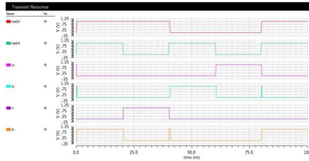
Fig 11. Output waveforms of 2x4 Decoder
