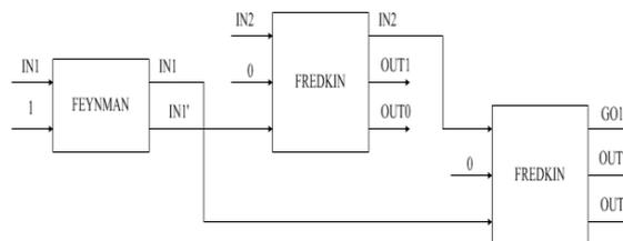
Fig 6. 2x4 Decoder using 1FEYNMAN & 2FDK gates
