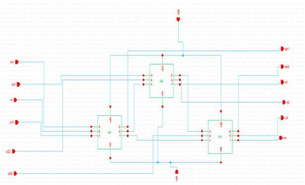
Fig.7 Schematic of Decoder using 1FEYNMAN & 2FDK gates
