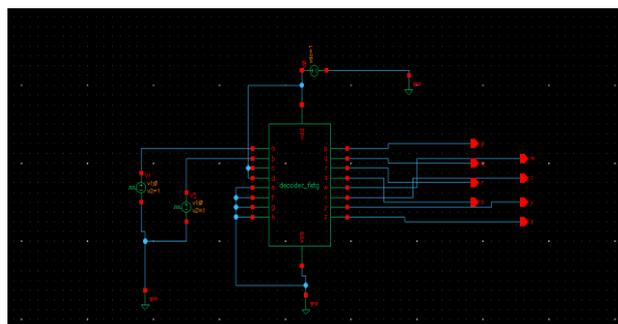
Fig 10. Test circuit for 2x4 Decoder using 1FEYNMAN & 2FDK gates
