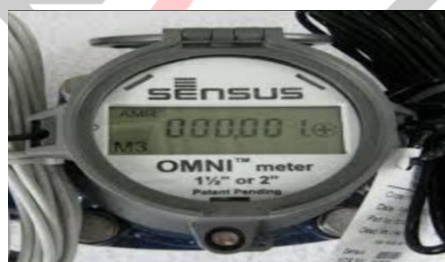
FIG.5. WATER FLOW METER
