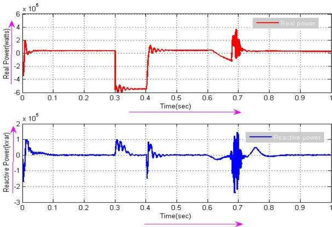
**Fig 12:Real and Reactive Power measured at the grid side at faulted condition without power smoothing system.**
