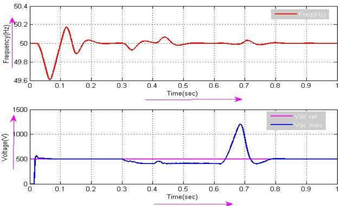
**Fig 10: Frequency and Vdc measured, Vdc reference voltage waveforms without power smoothing system.**
