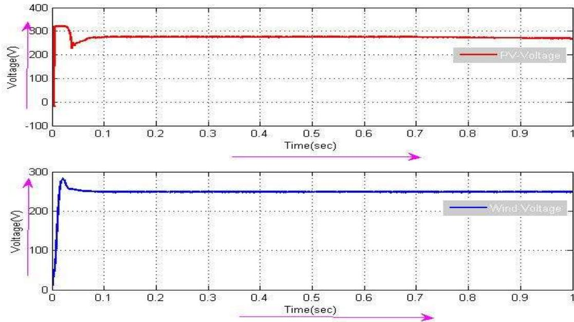
**Fig .7. Solar and wind voltage waveform with power smoothing system.**
