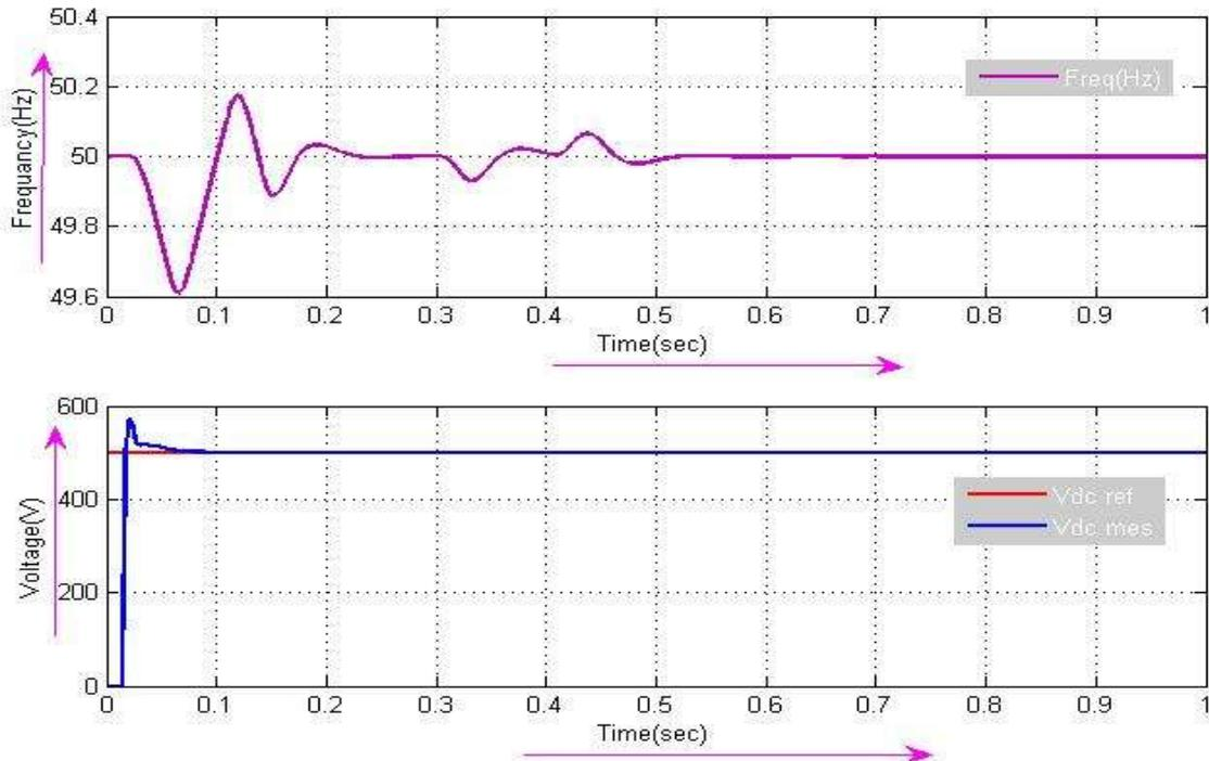
**Fig 9: Frequency and Vdc reference, Vdc measured voltage without power smoothing system.**
