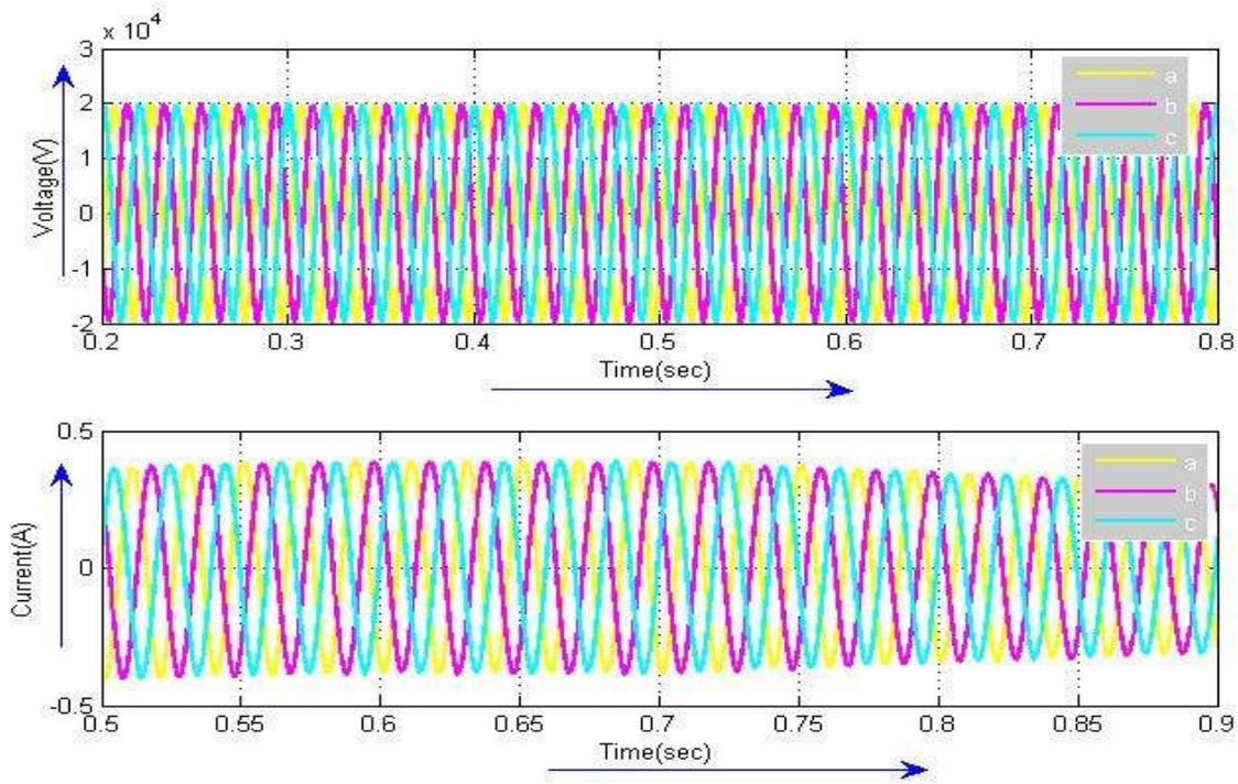
**Fig 13 Grid side Voltage(Vabc) and Current (Iabc) with Power smoothing system at faulted condition.**
