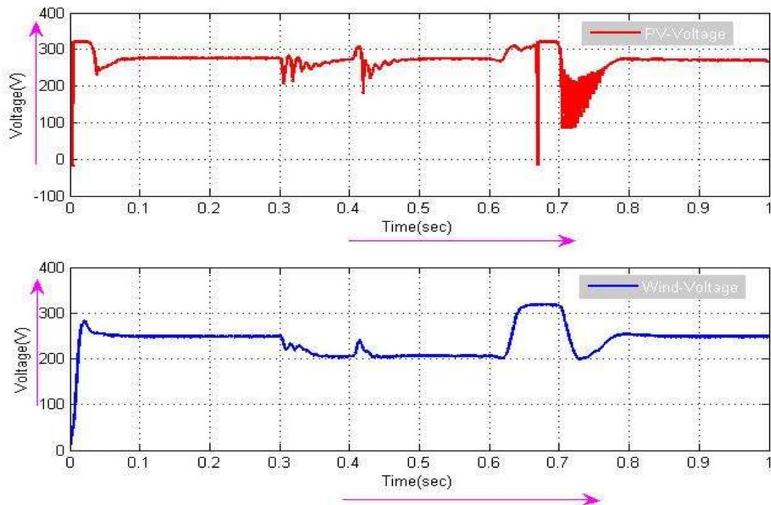
**Fig .8.Solar and Wind voltage waveform without power smoothing system.**
