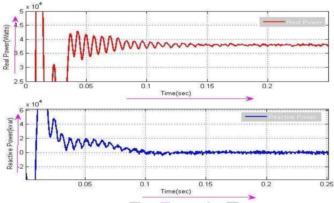
**Fig 11 Real and reactive Power Measured at the grid side at faulted condition with power smoothing system.**
