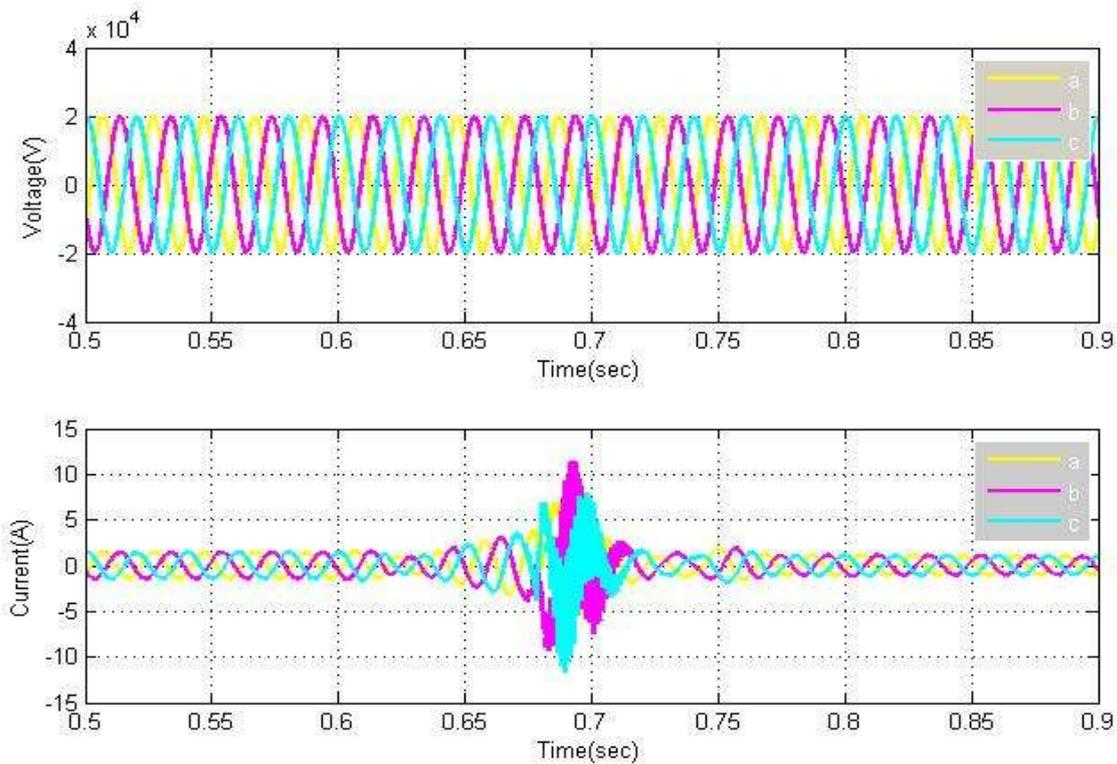
**Fig 14: Grid side Voltage(Vabc) and Current (Iabc) without Power smoothing system at faulted condition.**
