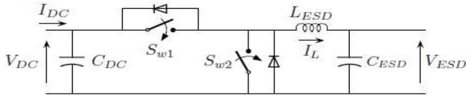
**Fig.2. Bidirectional topology used for ESS**
