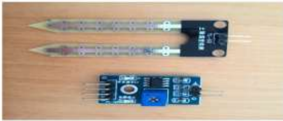
Figure:9.YL-69 moisture sensor.
