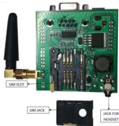
Figure.7. Rear view of GSM/GPRS module
