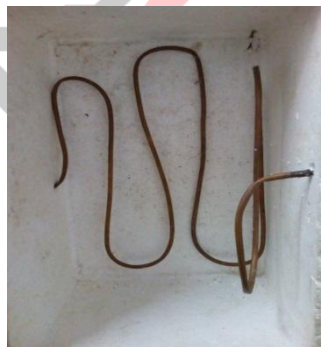
[Fig.14 Evaporative cooling coil]
