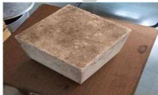
Fig7.2: Cube showing smooth surface
