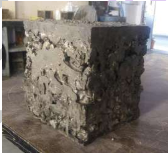
Fig.7.1: Cube showing rough surface
