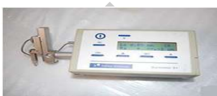
Fig 4 Talysurf tester for surface roughness measurement
