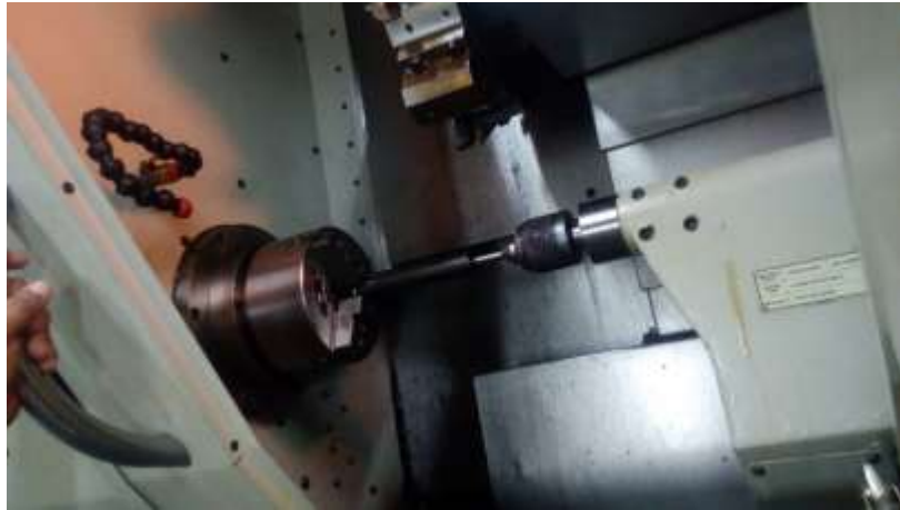
Fig 3Experimental set up in Harding SV150 CNC lathe machine
