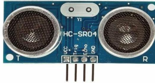
**Fig 3.1.**Ultrasonic sensor
