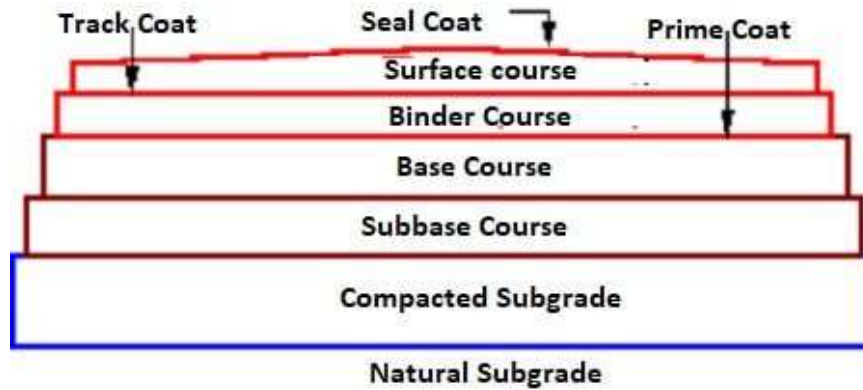
Fig 0.1: Typical layers of flexible pavement
