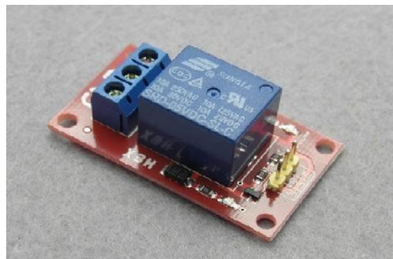
Figure No.15: Relay used to actuate gear dc motor
