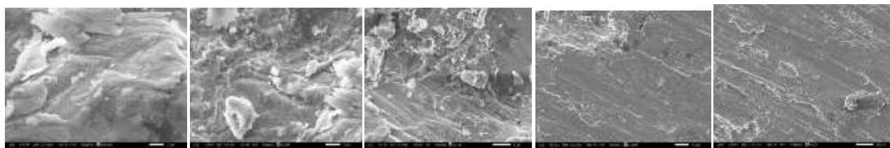
FIG 6.3 SEM IMAGES OF AL7075-B4C 5% MMC AT DIFFERENT MICRONS
