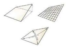
The structural strength of these roofs is attained by their curvature. Downward curvature along its section acts as an arch by absorbing the compressive stresses, hence to resist the thrust reaction exerted by downward curvature and their supports must be buttressed. Whereas the perpendicular curvature to the downward curvature undergoes tension or upward pull and hence must be reinforced to carry the tension (if built out of concrete).
