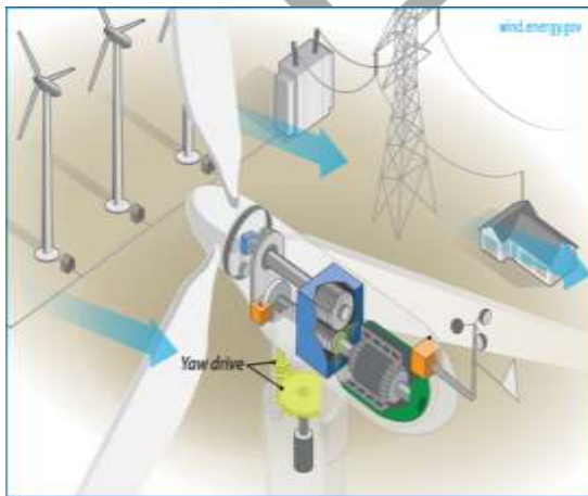
Fig 1: Detailed view of yaw drive
