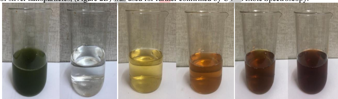
FIGURE 1: (A) Prepared Lantana camara leaf extract; (B) Prepared 1mM silver nitrate Solution; (C) Initial (pale yellow); (D) 10 minutes (deep yellow); (E) 30 minutes (brown); (F) 1 hour (dark brown)
