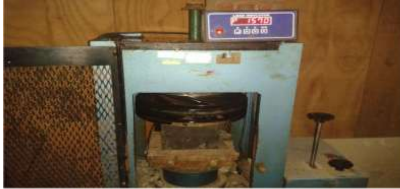
Figure 3.2 Test setup of compressive strength
