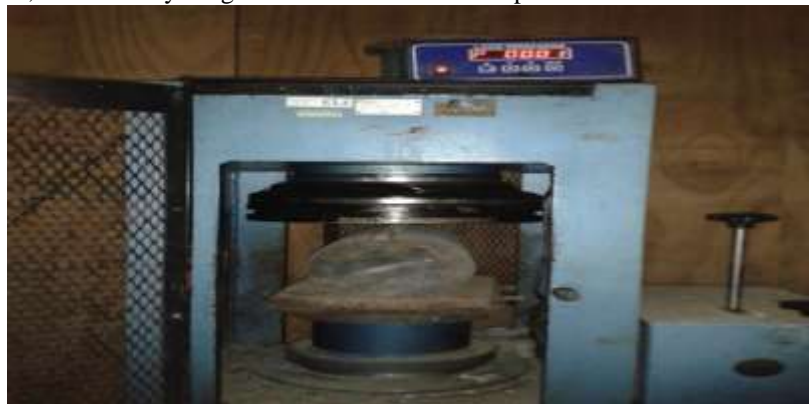
Figure 3.3 Test setup of split tensile strength
