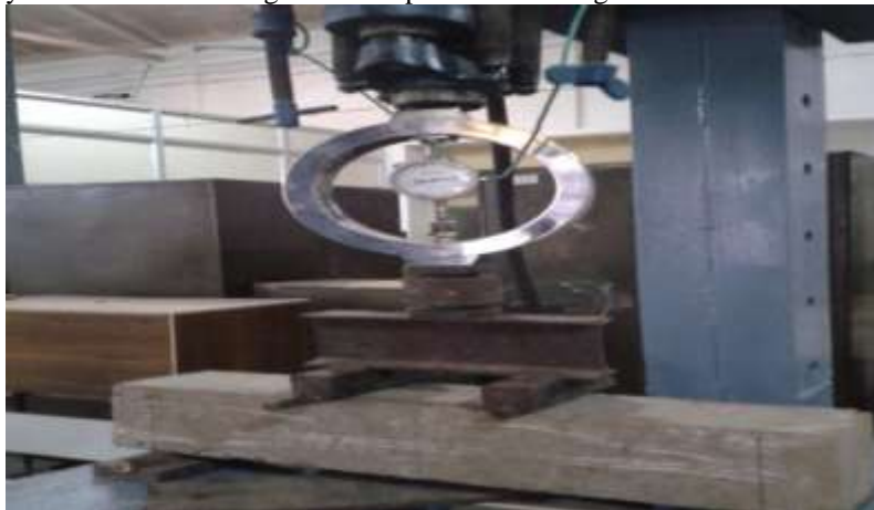
Figure 3.4 Test setup of flexural strength
