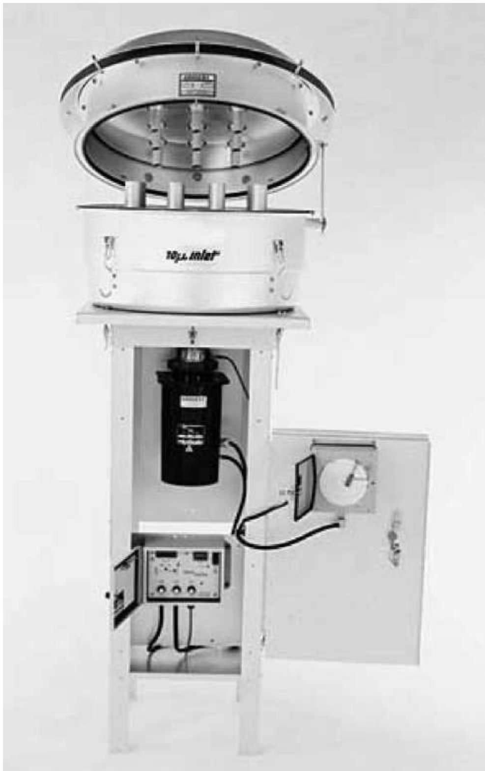
Fig. 11-5. Andersen PM10 high volume sampler.
