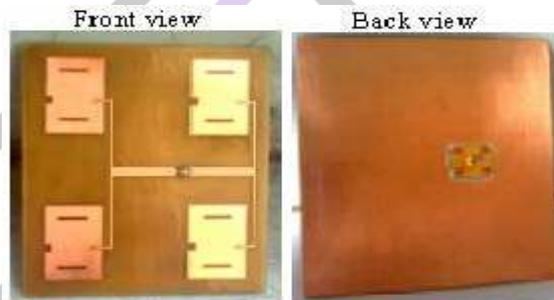
Figure 9. The prototype of the proposed array.
