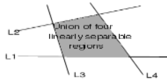
Fig 6: Intersection of 4 linearly separable regions forms the centre region
